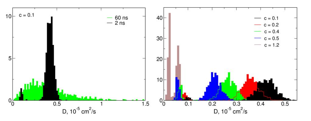
distributions of DME diffusion coefficients estimated in different time intervals for the c = 0.1 M electrolyte
