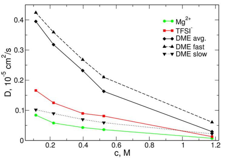
diffusion coefficients estimated from MD simulations for electrolytes with increasing salt concentration
