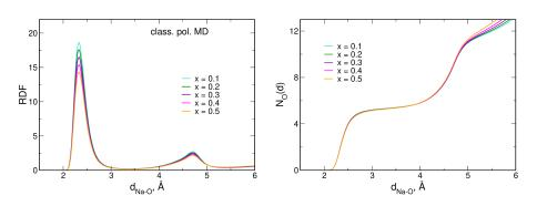
Na-O RDF and its integral obtained from polarizable FF classical MD
