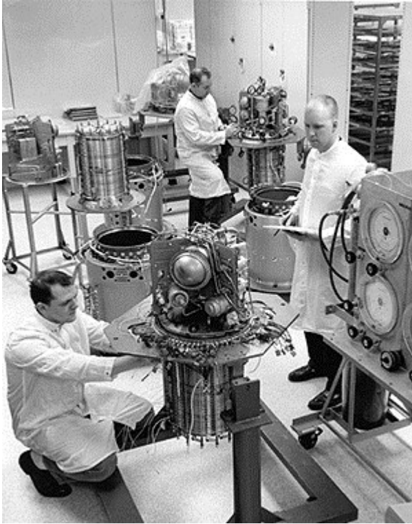
A Pratt & Whitney alkali fuel cell being assembled for an Apollo spacecraft, 1964
