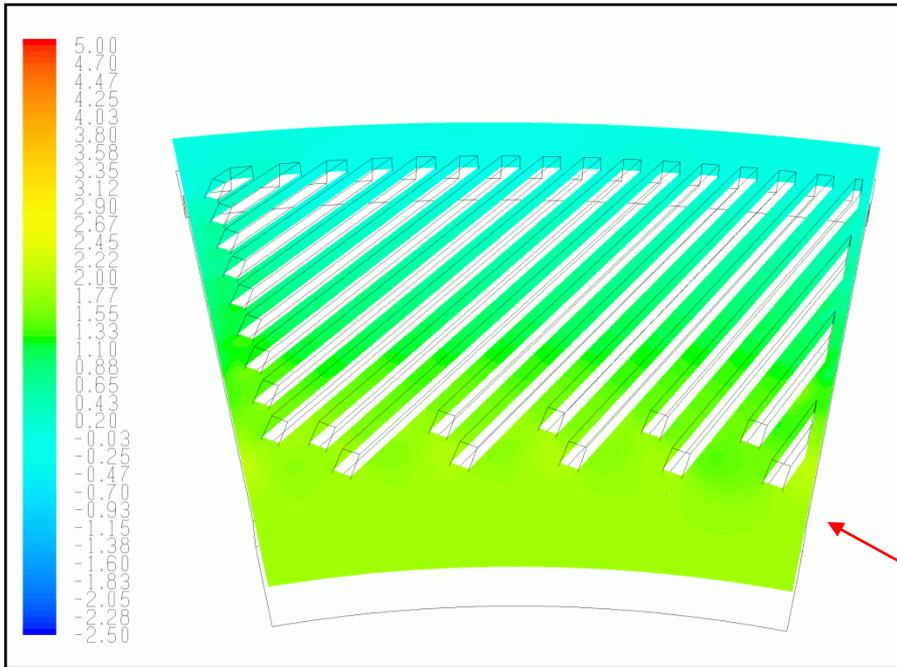
static pressure distribution [bar] at the centre of the stator bars
