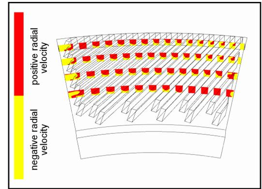
radial velocity at cross section at constant radius
