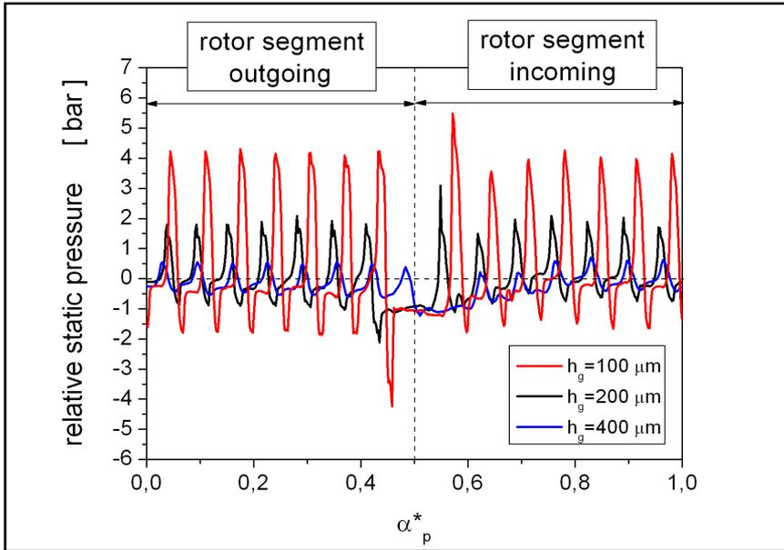
static pressure variation at the point loaded in the stator bar along with the phase shift
