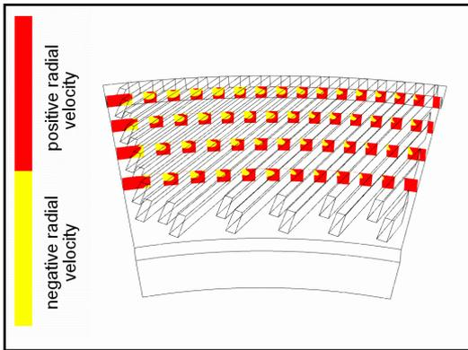
radial velocity at cross section at constant radius
