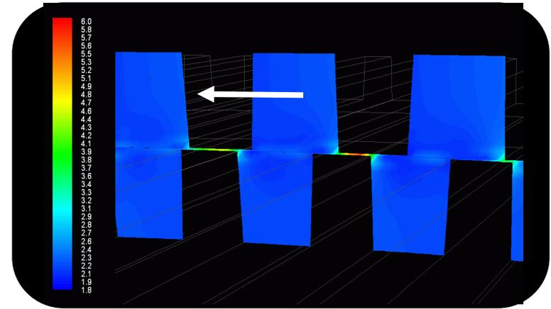
static pressure distribution [bar] at cross section through stator and rotor
