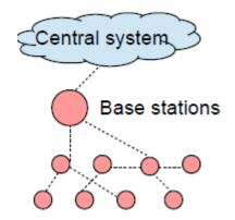
In the Edge Computing concept the data gathered by sensors can be processed close to the sensors and only selected preprocessed results can be transmitted to the central system
