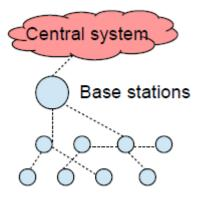
In a classical approach to WSN, the data gathered by sensors are transmitted usually through the mesh or tree topology to a central system for processing
