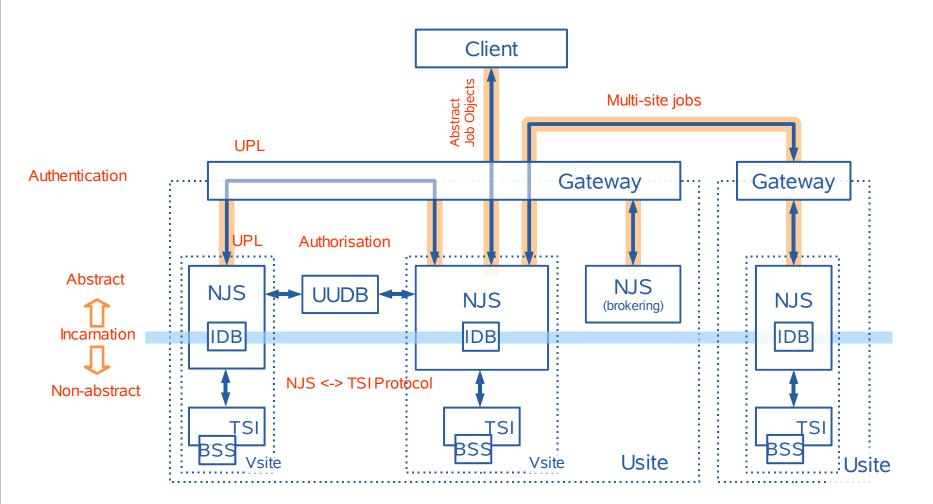
TSI – Target System Interface NJS – Network Job Supervisor IDB – Incarnation Database UUDB – UNICORE User Database Usite – UNICORE site UPL – UNICORE Protocol Layer
