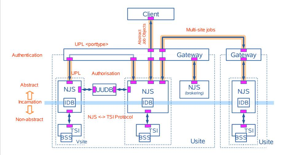
TSI – Target System Interface NJS – Network Job Supervisor IDB – Incarnation Database UUDB – UNICORE User Database Usite – UNICORE site UPL – UNICORE Protocol Layer Indicates SSL transport
